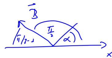
$$\begin{aligned}\vec{B} &= B (\cos(\frac{\pi}{2} + \alpha) \vec{i} + \sin(\frac{\pi}{2} + \alpha) \vec{j}) = \\ &= B (-\sin\alpha \vec{i} + \cos\alpha \vec{j})\end{aligned}$$
