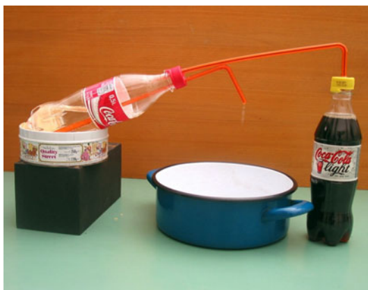
Figure 1. The \text{CO}_2 from the bottle on the right will replace all the water in the bottle on the left in a few hours.
