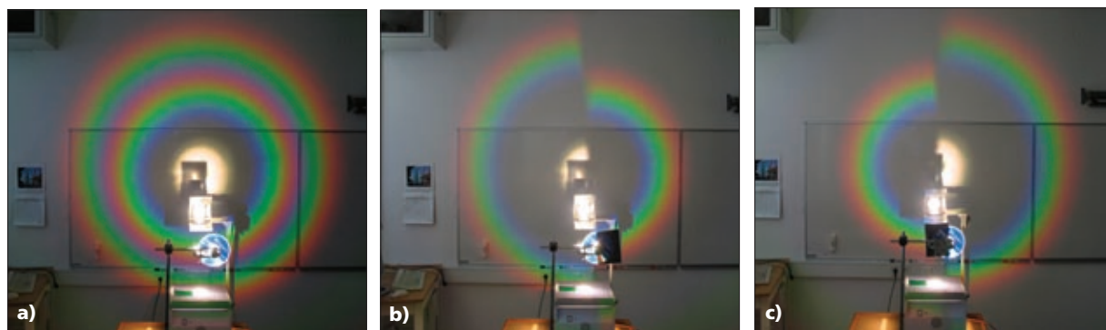
Fig. 1. (a) Rainbow-like spectrum caused by light reflection from a CD. (b) Spectrum obtained when the right-hand side of the CD is blocked with an opaque card. (c) Spectrum obtained when the left-hand side of the CD is blocked with an opaque card.
