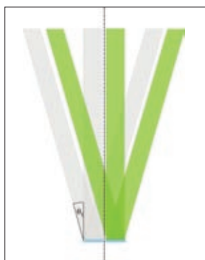
Fig. 3. Two sets of diffraction maxima (zero and first order) are formed in the plane through the CD diameter when monochromatic light is incident on a CD. For clarity, one set is shown in gray.
