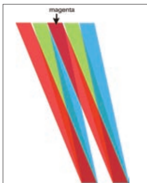
Fig. 4. The appearance of a magenta color in CD “rainbow.” For clarity, only the red-green-blue light components and only half of the first-order maxima are shown.
