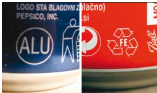
Figure 5. Labels on soda cans that indicate the type of metal: aluminium (left) and steel (right). Note that the design of the labels may vary.
