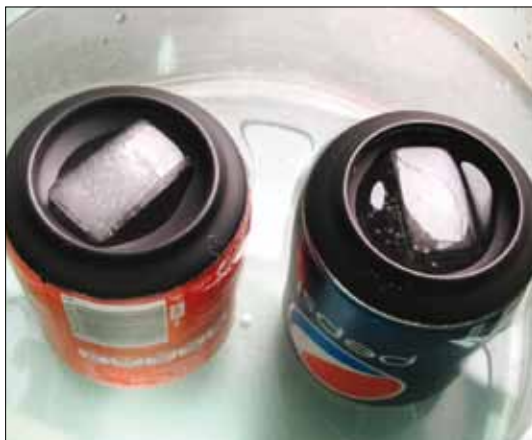
Figure 4. The ice cube on the Pepsi can (right) is melting faster than the ice cube on the Coke can (left). The can bottoms are sprayed black to improve the visibility of the melted ice.
