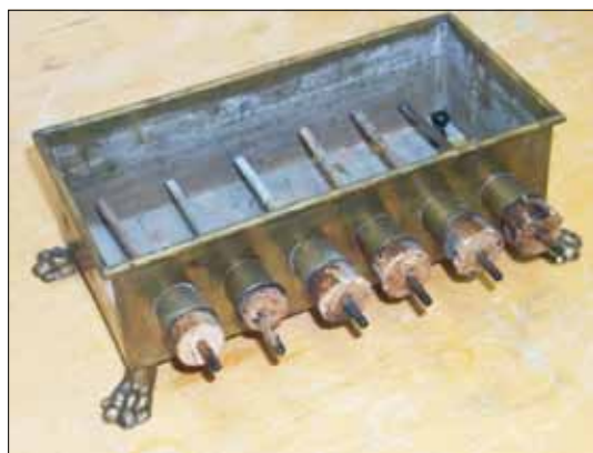
Figure 1. Old demonstration experiment for comparing thermal conductivities of different metals (from the collection of Jurij Vega High School, Idrija, Slovenia).
