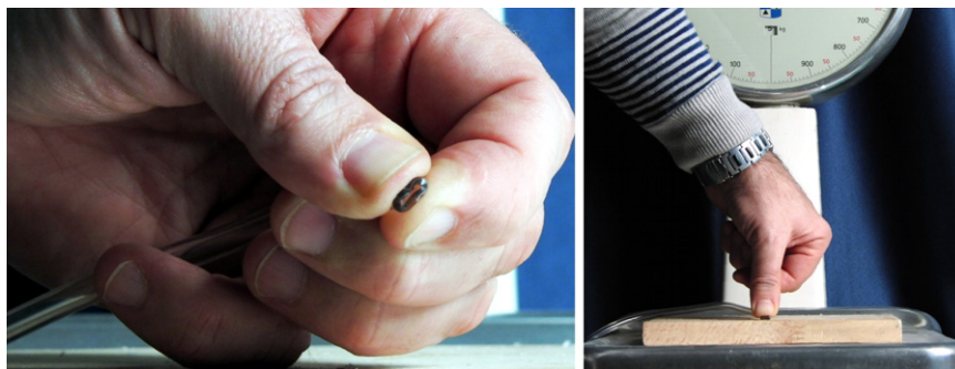
Figure 4. Tubing force meter. Tubing is first compressed by the fingers in a similar position as when shooting the pit (left). After that the same deformation is achieved by pressing the tubing on the scales (right).
