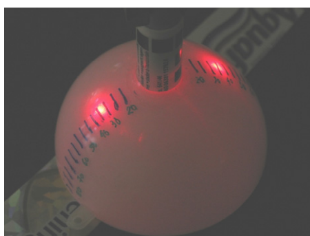
Figure 3. Diffraction patterns produced by the shiny part of a toothpaste package using red and green laser light respectively.
