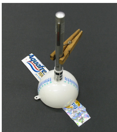
Figure 2. Safe Laser Inspection Device made from one hemisphere of a painted Christmas ball.
