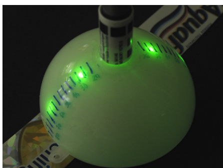
Figure 3. Diffraction patterns produced by the shiny part of a toothpaste package using red and green laser light respectively.
