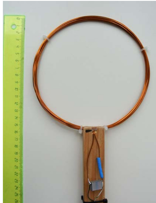
Figure 7: The photo of the resonant circuit used in the experiment
