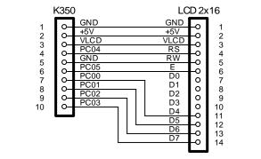
Figure 1: The connection of the liquid crystal display using a four but data-bus and two-bit control bus
