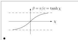
The control points of the two Bézier curves were calculated with formulas (5.1). The positive branch is determined by  $P_1 = (0, 0), m_1 = 1$  and  $P_2 = (2, \tanh 2), m_2 = 1/\cosh^2 2$ . Again, the picture is defined in mathematically convenient coordinates, and the lower left corner is assigned the mathematical coordinates (-3, -2) (black disk).
